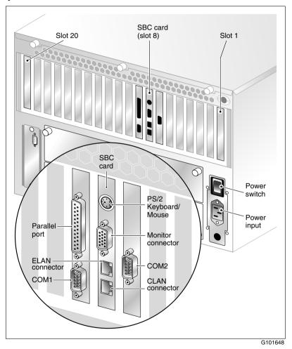
**Note:** The above diagram shows the power switch and power input for an AC server. The rest of the diagram is the same for AC or DC servers. For peripheral device connections, this picture applies to AC and DC servers.
